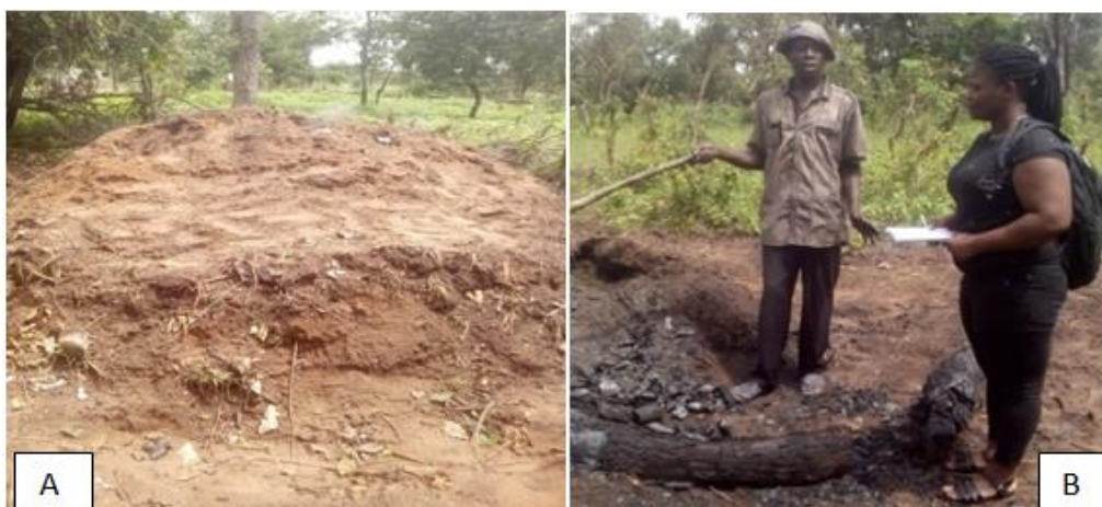
Figure 5: Earth-mound kiln Charcoal production site in Tse Taki Villge in Makurdi LGA (A) Sorting of charcoal from earth-mound kiln in Tse Umenger village in Guma LGA (B)
