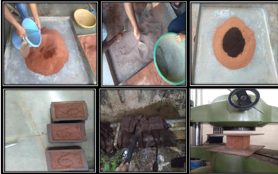
Fig. 3: Preparation of stabilized soil blocks
