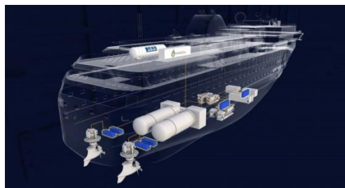
Fig 4: Illustration of hydrogen propulsion systems with integrated LH 2 tank and fuel cells [11]
