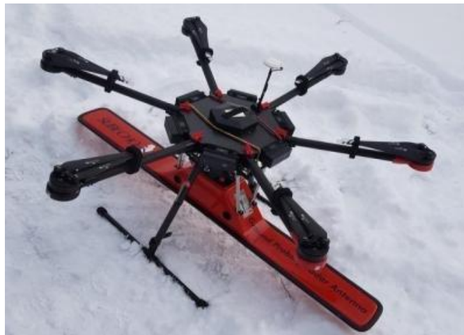
Fig 2. GPR drone (DJIM 600 pro) integrated system
