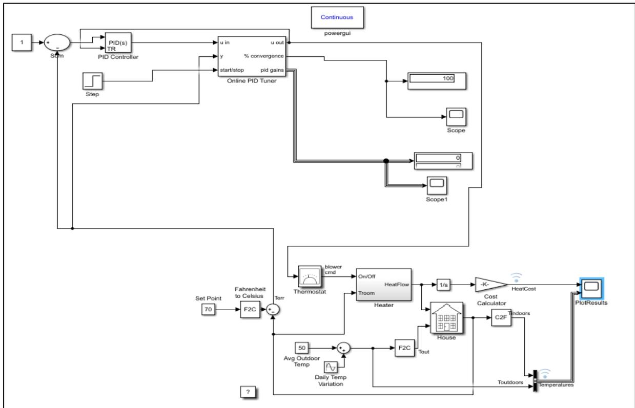
Fig. 3 Simulink model of PID Auto tuner with HVAC
