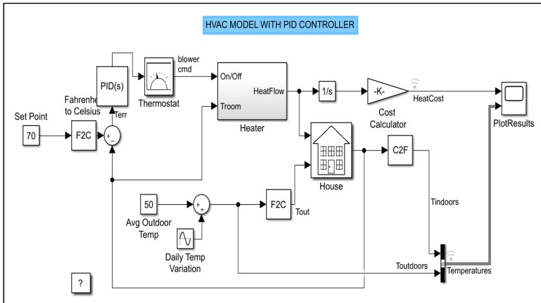
Fig. 1 Simulink model of PID controller with HVAC System
