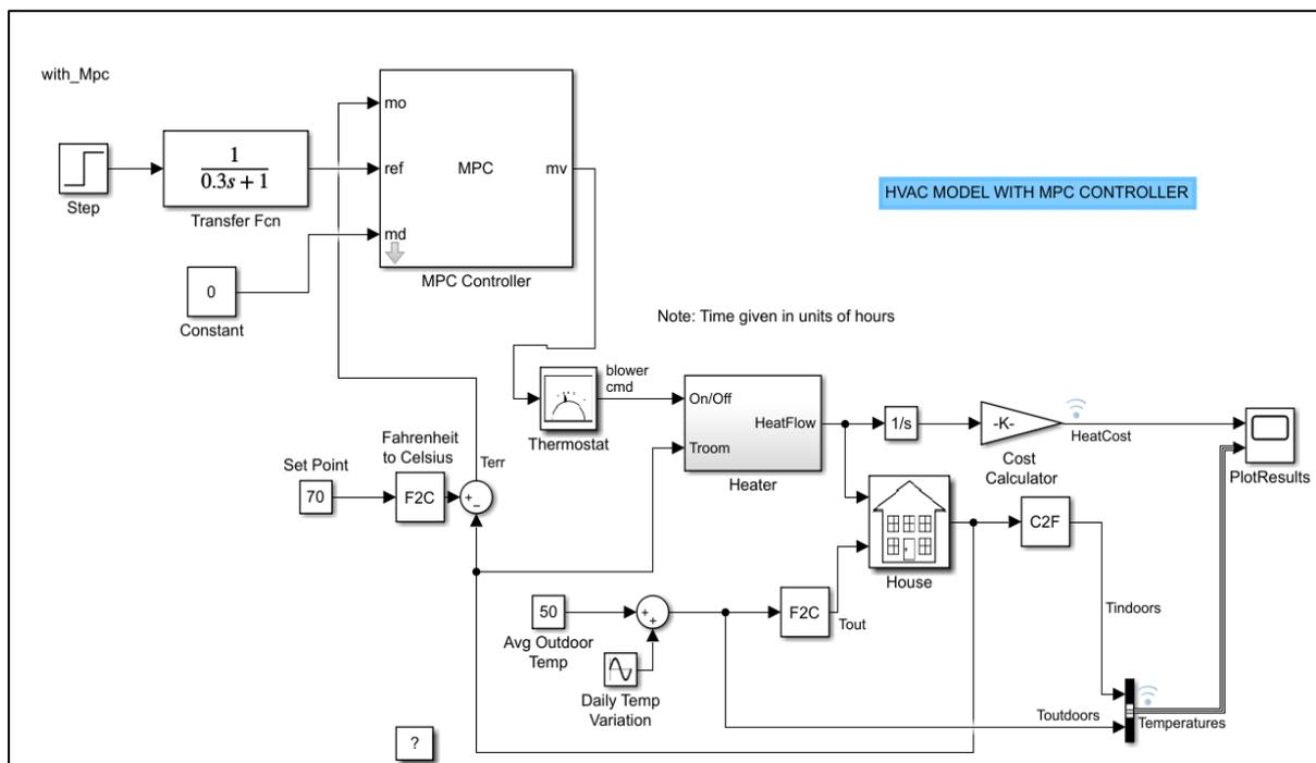
Fig. 2 Simulation model of MPC controller with HVAC
