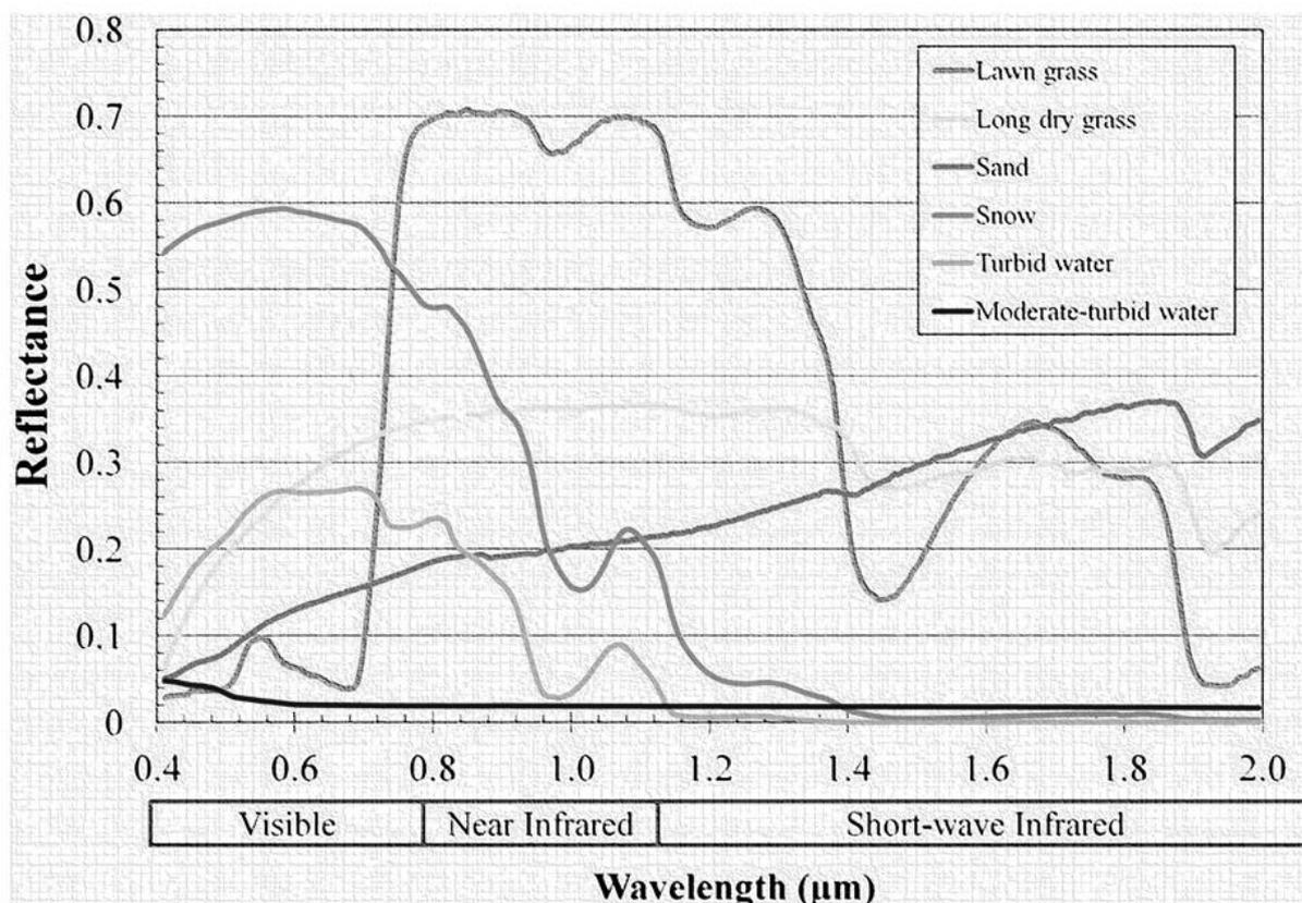
Fig. 2: The reflectance of several typical land cover objects, collected from the United States Geological Survey (USGS) digital spectral library (<https://speclab.cr.usgs.gov/spectral-lib.html>)
