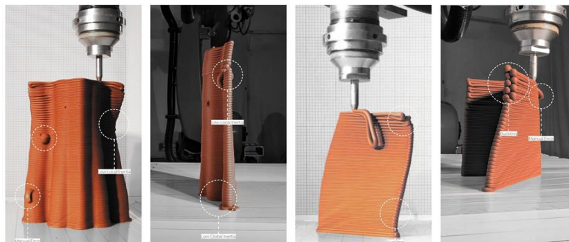
Fig 4: Test prints to analyze structural parameters (Datta et al., 2019)
