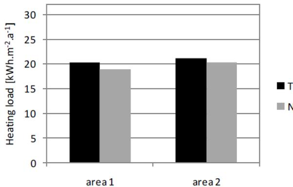
Fig. 6. Comparison of heating loads between area 1 & 2 (present climate) (Source: EnergyPlus Version: 22.1.0)
