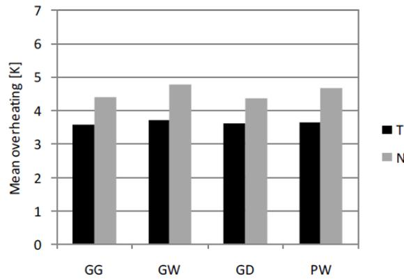
**Fig. 10.** Mean overheating, area 1, present climate (Source: EnergyPlus Version: 22.1.0).
