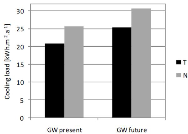
**Fig. 9.** Comparison of present and future cooling loads (area 1) (Source: EnergyPlus Version: 22.1.0)
