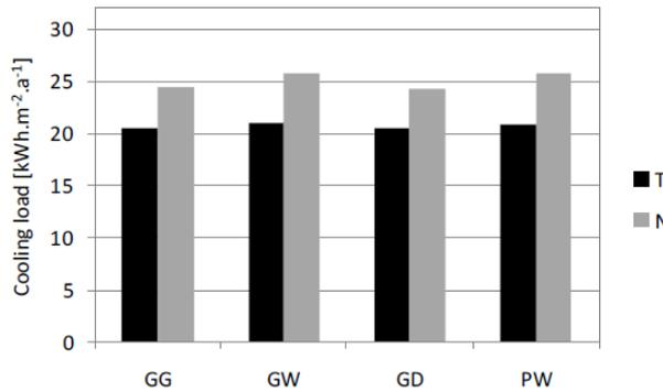
Fig. 5. Cooling loads, area 1, present climate (Source: EnergyPlus Version: 22.1.0)
