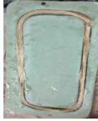
Figure 1: GFRP stirrup casting in mold with GFRP fibers
