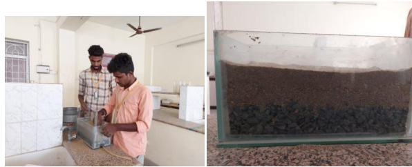
FIG. 5 - Setting Up the Conventional Sand Filter
