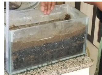
FIG. 6 - Setting Up the Modified Sand Filter
