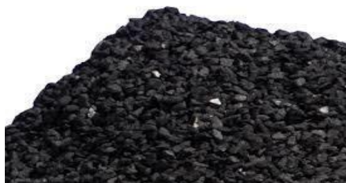
FIG. 1 - Granular activated carbon
