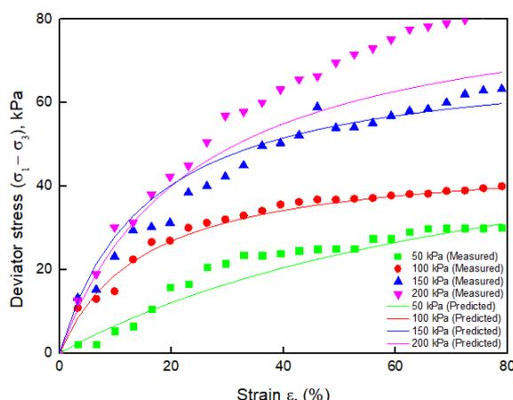
Fig. 7 Comparison of measured and predicted stress – strain curves for soil sample with 37.22 % moisture content
