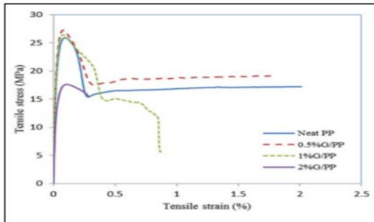
Fig 4: Stress strain curve of polypropylene mesh [12]
