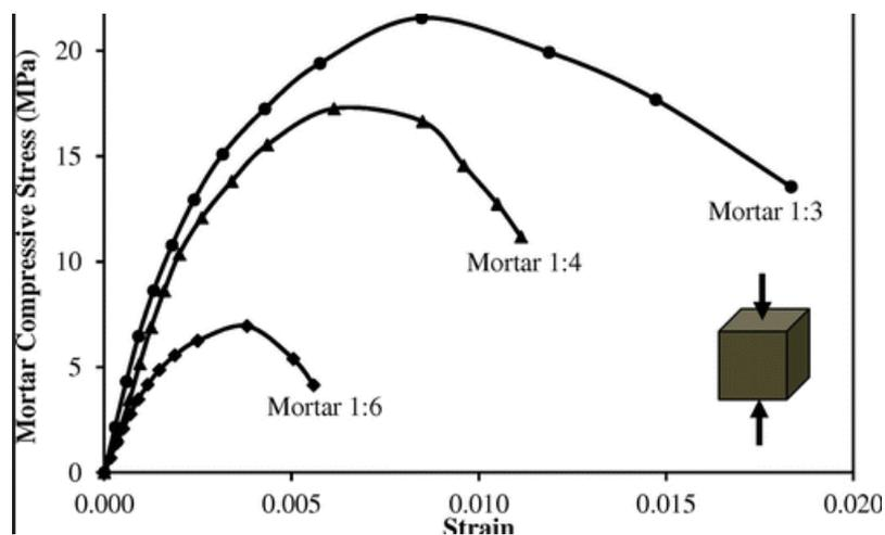
Fig 3: Stress strain curve of mortar with compressive strength of 20 MPa[11]
