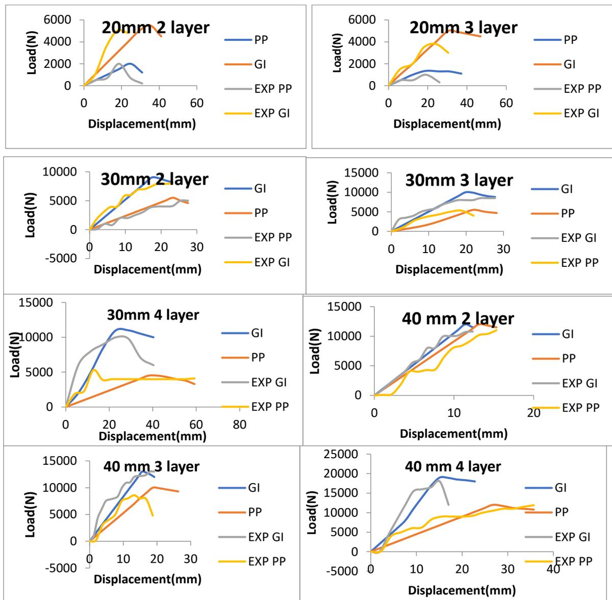
Fig 7: Load deformation responses from numerical analysis
