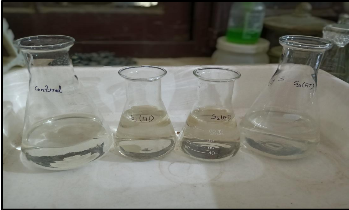
Fig- 4 Water samples after 3 weeks of Treatment -1. Control, 2. Sample 1(STP water inoculated with 50 g of A.pinnata ), 3. Sample 2(STP water inoculated with 100 g of A.pinnata ), 4. Sample 3(STP water inoculated with 150 g of A.pinnata ).
