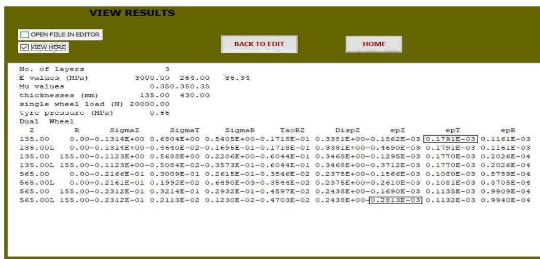
Fig. 5. Output screen of IITPAVE software for pavement system modeled for CBR 12%
