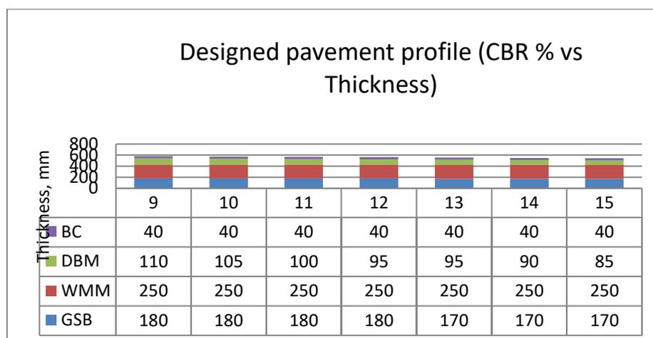
Fig. 3. Variation in the thickness of pavement system with CBR value (9% to 15%)
