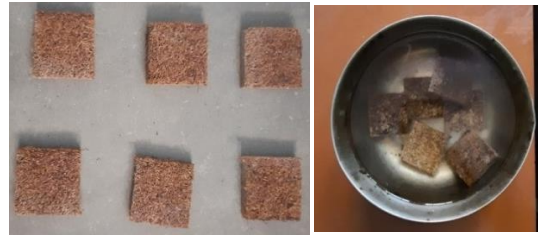
Fig. 2 Test samples for water absorption and thickness swelling tests
