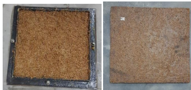
Fig. 1 Particle board before and after compaction
