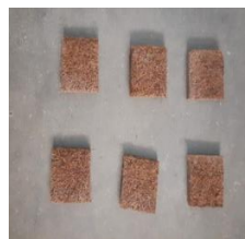
Fig. 3 Test sample for flexural strength test
