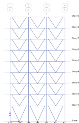
Fig.4 Model 4: V bracing Diagonal with 10% eccentricity 10%
