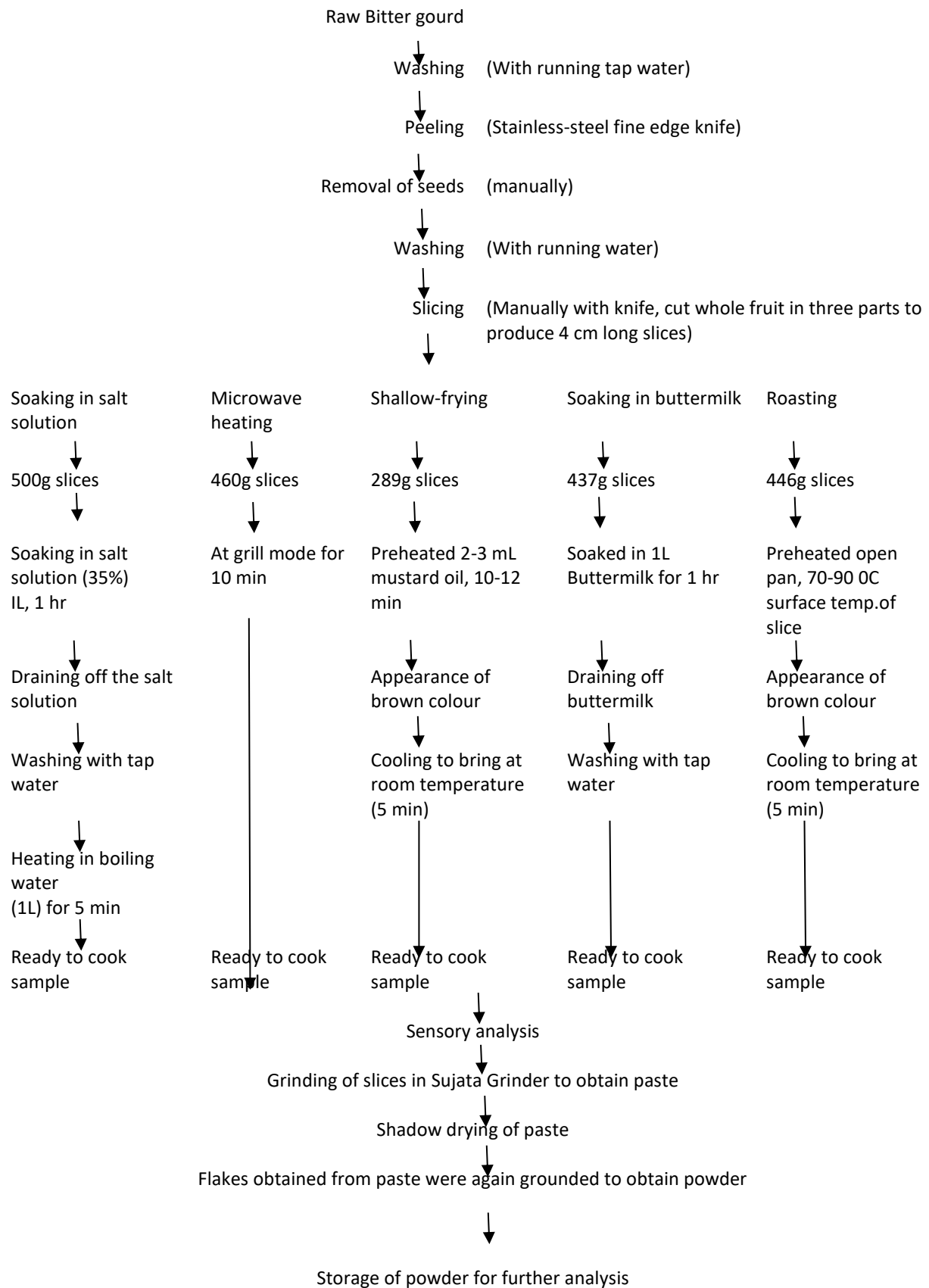
Fig. 1 Process flow diagram for processing of Bitter Gourd
