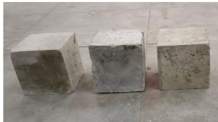
Fig.3 Cubes of control mix
