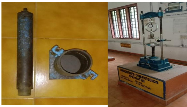
Fig. 1 Proctor's cylindrical mould and base plate Fig. 2 UCS Apparatus
