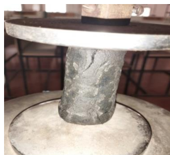
Fig 4. Crack formation during UCS test
