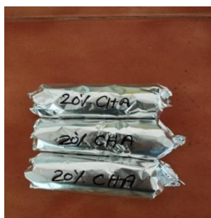
Fig 1. Soil specimen get wrap with foil paper
