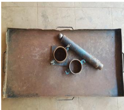
Fig.1. Proctor cylindrical mould, base plate and hammer Fig.2 UCS Apparatus
