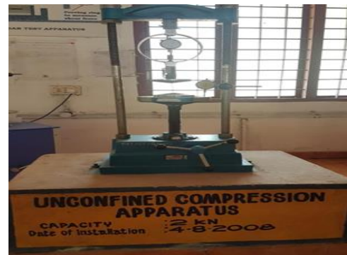
Fig.1. Proctor cylindrical mould, base plate and hammer Fig.2 UCS Apparatus
