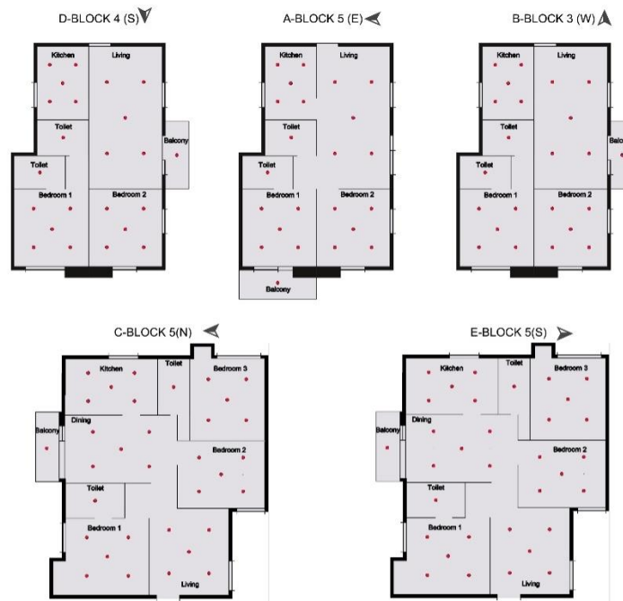
Fig. 7 Indoor measuring point
